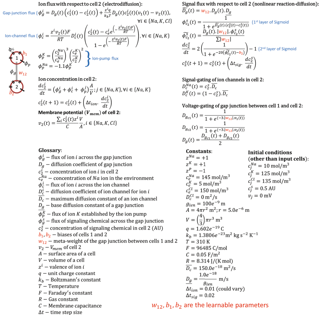
Figure 8. Mathematical details of the BEN model. (Top) The equations that describe the dynamics in a 2-cell system illustrated in the figure on the left. (Bottom) A glossary of variables used in the equations, the constants and initial conditions.
