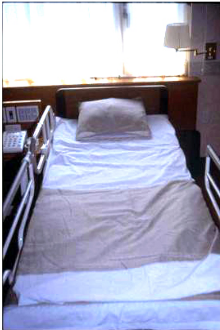
Fig. (3). Bed monitoring system. The electroconductive material was woven into the bed sheet. The pillow and lower part of the sheet shown by the dark colour in the photo are connected to two ECG electrodes.
