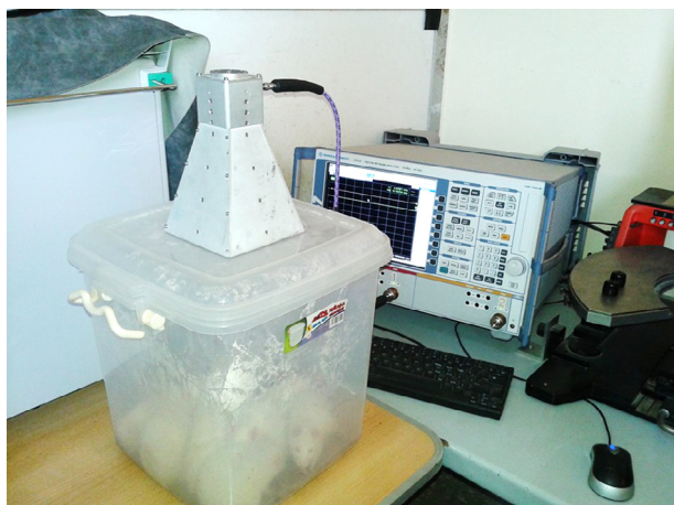
Fig. 1. Microwave generator with microwave analyzer (ROHDE & SCHWARZ ZVA67 vector network analyzer 10 MHz–67 GHz - USA). The electromagnetic waves signals generate a radiation frequency at 900 MHz. mimicking mobile phone, and the electromagnetic waves were radiated through horn antenna to caged rats.
