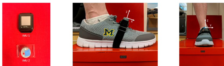
Figure 1. Two inertial measurement unit (IMU) designs and the means of attachment to a foot. (a) IMU 1 (Opal, APDM, left) and IMU 2 (custom design, Insight Sports, Ltd., right); (b and c) Side and front views of attachment of both IMUs to the instep via a Velcro strap. Sensor axes are denoted by X, Y, and Z (X and Z largely lie in foot sagittal plane and Y largely points to subject's left). Note that these axes are illustrated to aid interpretation of the raw data signals presented in Figures 4 and 8, and that the zero-velocity update (ZUPT) method herein does not require specific sensor alignment to anatomical axes.
