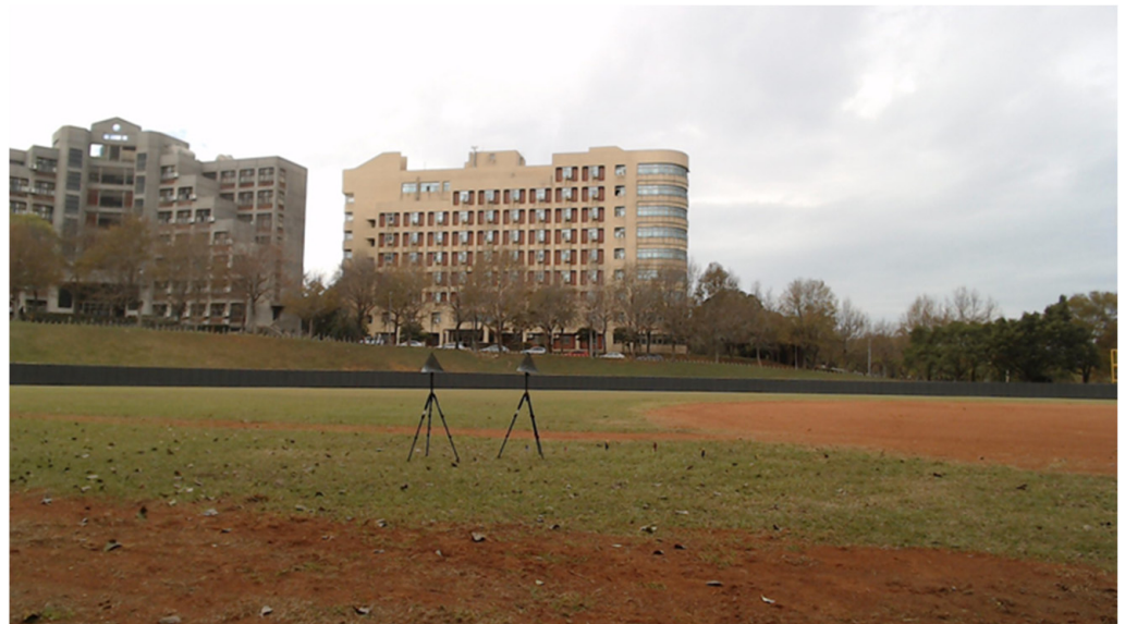
Figure 5. Experiments with two metal corner reflectors (targets).
