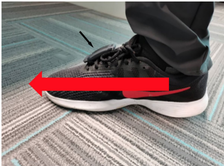
Fig. 2. The placement of the IMU on the shoe: the black arrow points to the IMU, the red arrow points to the longitudinal axis of the foot.
