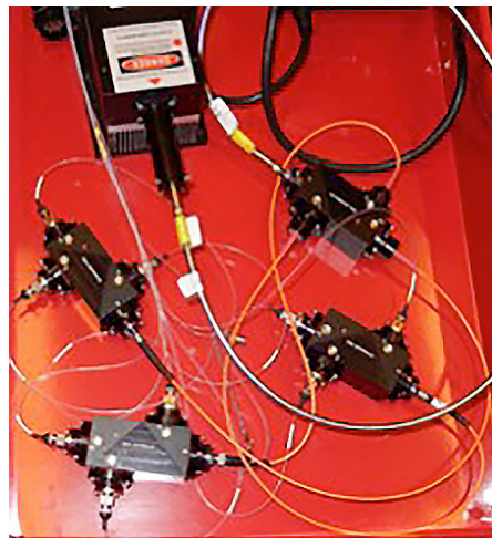
Figure 2. Infrared laser heating system. A main optical fiber for moderate heating connects to a primary three-way splitter box. Three secondary splitter boxes connect via three separate optical fibers to the primary three-way splitter box (orange fibers). Each of the three secondary splitter boxes directs the laser beam through three optical fibers connected to the main optical fiber. Shutter control is performed manually by nine individual shutters.
