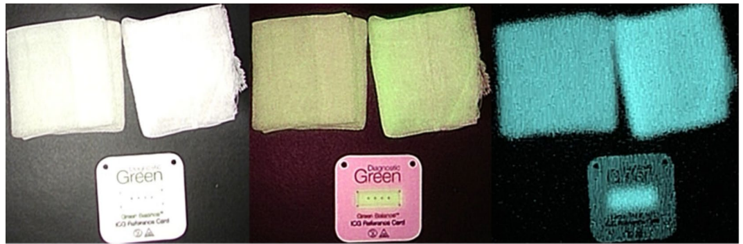
Fig. 6. A fluorescent gauze dyed with a 100-fold diluted pure ICG solution was stored under light-shielded conditions and maintained stable fluorescence intensity for over three years. Left: newly prepared gauze. Right: gauze prepared three and a half years ago. A, white light. B, NIR light in magenta mode. C, NIR light in monochrome mode.
