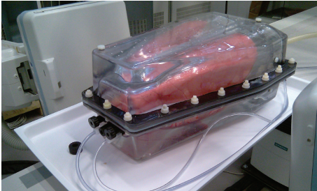
FIGURE 8: Illustration of the artiCHEST lung phantom. The box contains a porcine lung mounted on an artificial diaphragm and is filled with water.
