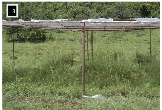
Fig. 1. (A) The layout of rainfall manipulation plots. Parallel arrows show transparent rainout gutters used to simulate rainfall reduction and direction to which excluded rainfall flows (rainfall increment plot/150% rainfall). (B) Photograph of rainfall manipulation plot with a slanted roof partially covered by transparent rainout gutters to exclude 50% of the rainfall and redirect it to the plot designated to receive more rainfall (i.e., 150% rainfall).
