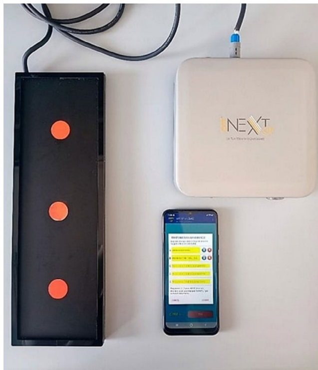
FIGURE 2 | The CMFs device (Next SX version; Medicina Fisica Integrata M.F.I., Rome, Italy) is equipped with a CMF generator, a support structure for cell plates and flasks, and a smartphone that runs the MFI-IP software (version 5.0; Medicina Fisica Integrata M.F.I., Rome, Italy), which is used to program the CMF generator. Source: This figure is derived from the research conducted by Gallorini et al. [37].
