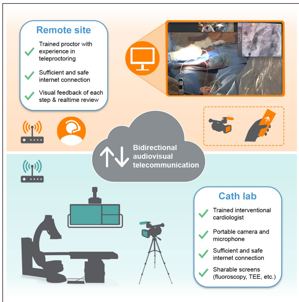
Figure. Illustration of used teleproctoring setup. TEE indicates transesophageal echocardiography.
