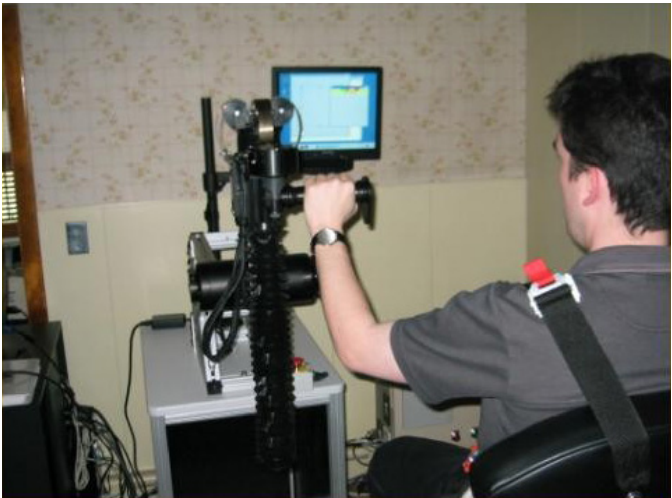
Figure 9 Vertical 1-dof Module Using Electrical Linear Technology. This commercial version of MIT's module can be operated in standalone fashion or integrated to the planar MIT-MANUS to allow spatial movements. Note that in the standalone fashion it can be operated at any angle to the horizontal and vertical planes with adjustable handle positions.
