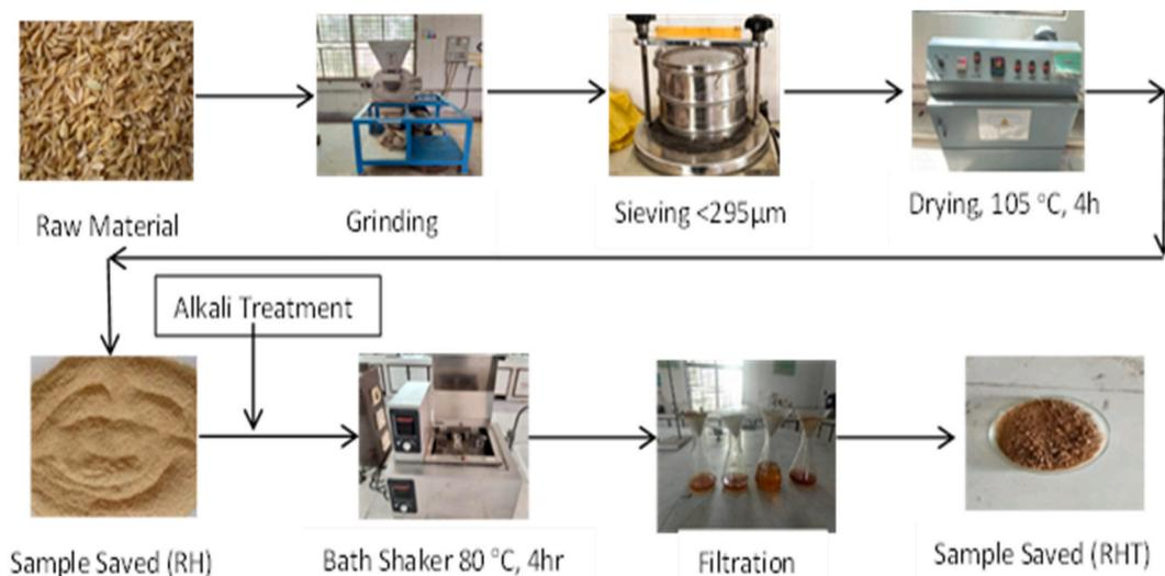
Fig. 1. Schematic Diagram for Physio-Chemical Pretreatment of Biowaste Rice Husk.
