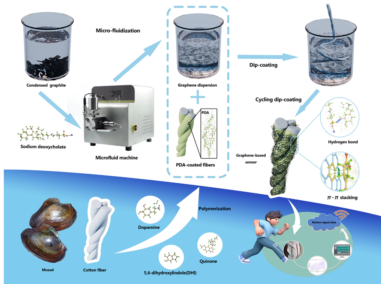
Figure 1. A schematic illustrating the production of graphene sensors based on polydopamine (PDA) and their integration in e-textiles for healthcare monitoring
