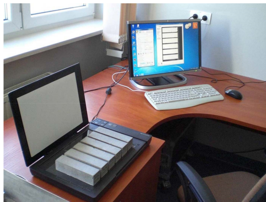
Figure 1. Test stand for scanning the surface of cement paste.
