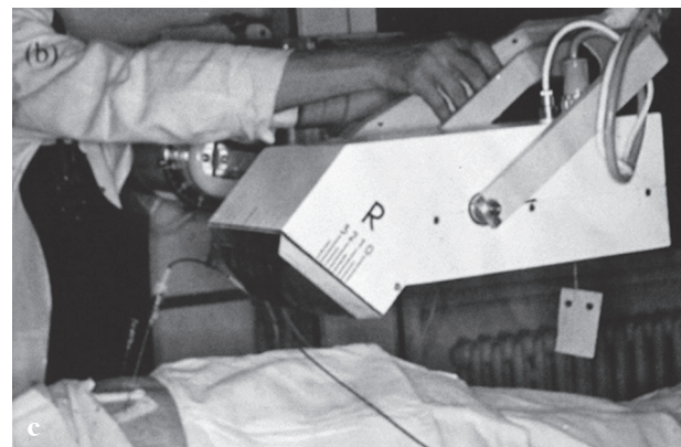
Fig. 8. — The Vidison was the first real time scanner and was popular in Germany. The frame rate was slow, the resolution poor but Manfred Hansmann (a) pioneered ultrasound guided intrauterine therapy (b) with this equipment (c).
