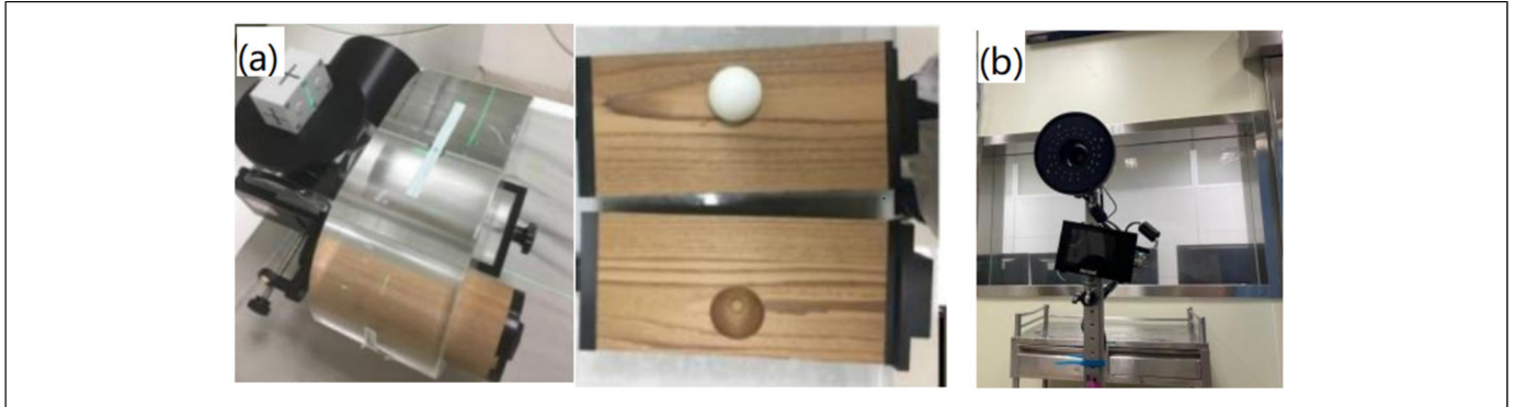
Figure 1. (a) QUASAR™ phantom with a ball inside simulating the tumor; (b) RPM system.
