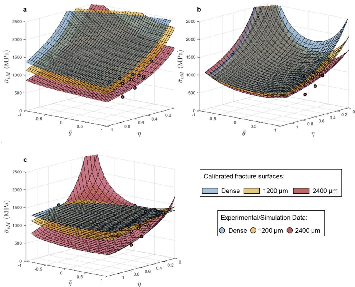
**Figure 7.** Calibrated (a) maximum stress, (b) Mohr–Coulomb, and (c) Hosford–Coulomb fracture loci in stress triaxiality vs. Lode angle parameter vs. equivalent stress space for Ti-6Al-4V using dense, 1200  $\mu\text{m}$  pore, and 2400  $\mu\text{m}$  pore data.
