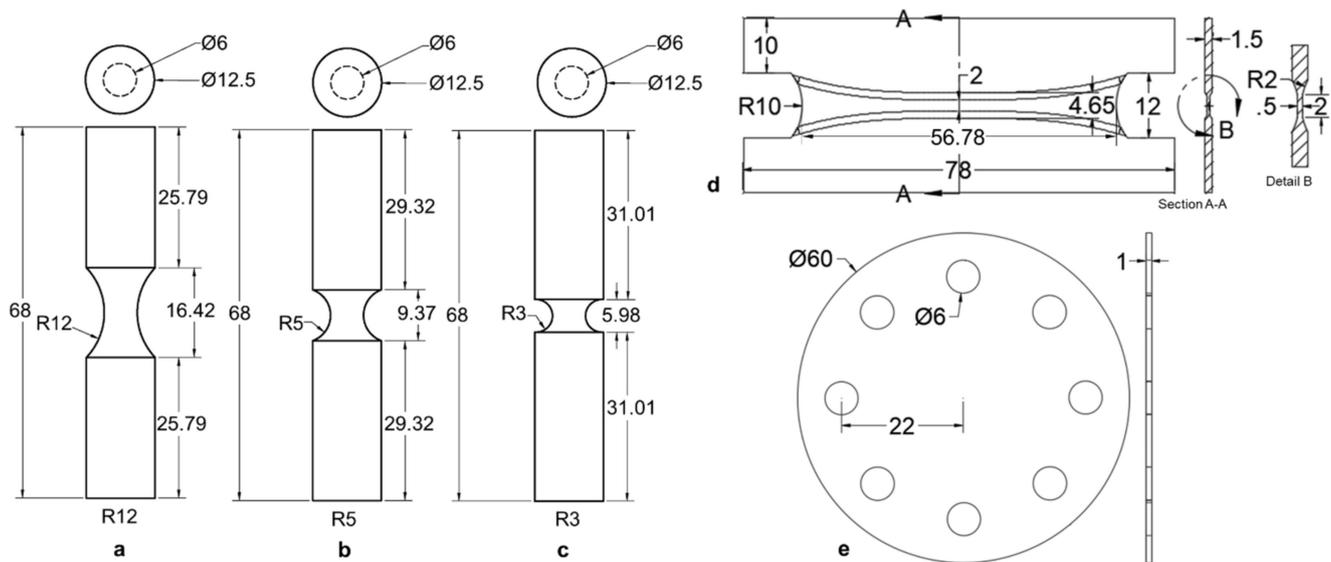
**Figure 2.** Drawings of mechanical test specimens used to calibrate fracture criterion. (a–c) The cylindrical notched tension geometries that were tested in the dense condition and with single, penny-shaped pores of varying diameter at the center. (d) The butterfly test geometry used to evaluate material properties under pure shear and (e) the punch test geometry used to evaluate equibiaxial tension. Both (d,e) were only tested in the dense condition. All dimensions in mm.
