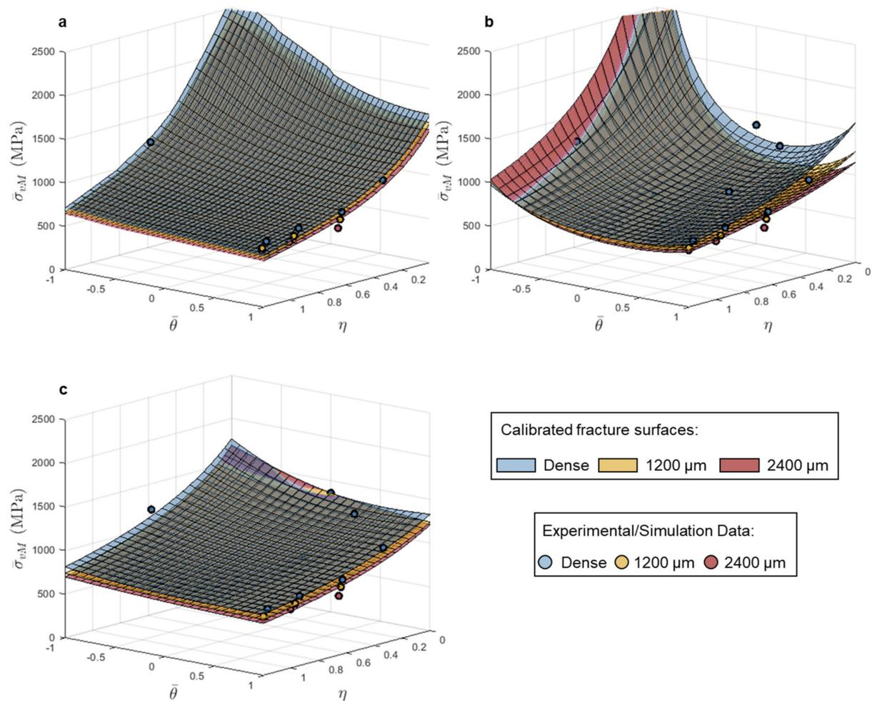
**Figure 6.** Calibrated (a) maximum stress, (b) Mohr–Coulomb and (c) Hosford–Coulomb fracture loci in stress triaxiality vs. Lode angle parameter vs. equivalent stress space for 316L using dense, 1200  $\mu\text{m}$ , and 2400  $\mu\text{m}$  pore data.
