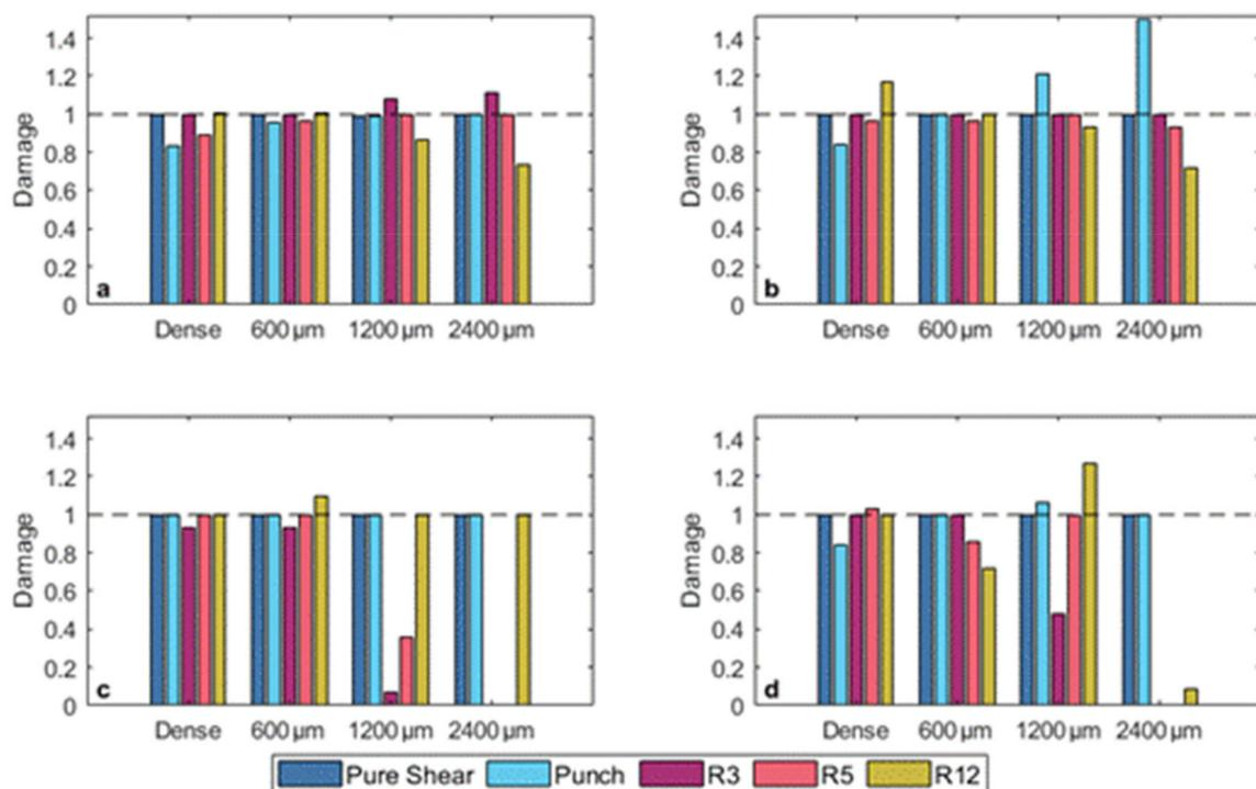
**Figure 3.** Damage accumulation at fracture for (a,b) 316L and (c,d) Ti-6Al-4V using the calibrated (a,c) modified Mohr-Coulomb and (b,d) Hosford-Coulomb models. The dashed line at a value of damage equal to one represents perfect agreement between the model and the experimental/simulation data for each test. Numbers on the horizontal axes denote the pore diameter at the center of the samples.
