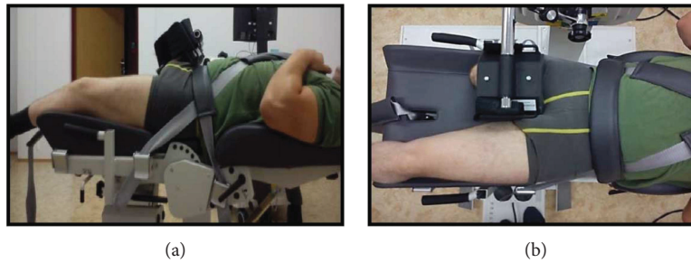
FIGURE 2: Test position for the hip flexor and extensor muscles. Side and top view.
