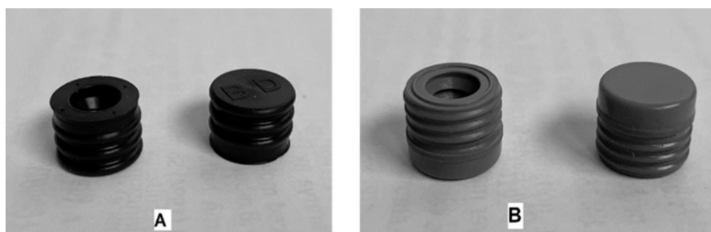
Figure 2. Pictures of the sealing pieces used in this study. Key, elastomer PH 701/50 C BLACK coded as JEA (A) and elastomer 4023/50 GRAY coded as JEN (B).
