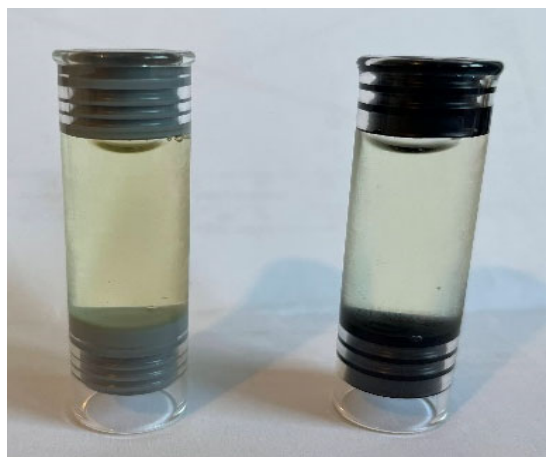
Figure 1. Example of the two sealing elastomeric gasket pieces (black colour right one and grey colour left part of the figure) located in the glass syringes.
