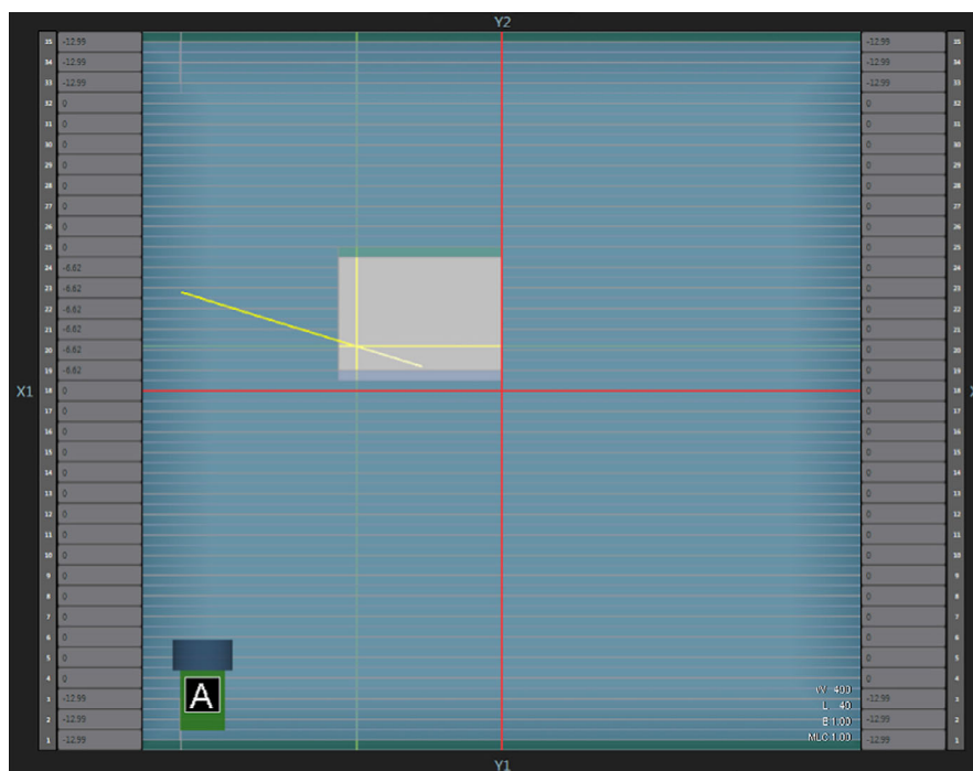
FIG. 2. Off-axis multileaf collimator aperture created in the treatment planning system. [Color figure can be viewed at wileyonlinelibrary.com ]
