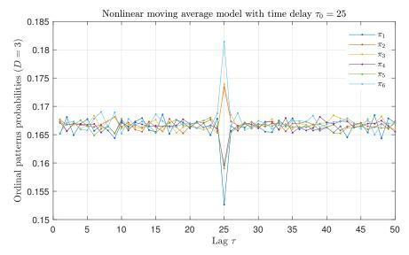
**Figure 2.** Ordinal patterns probabilities with D=3 as a function of the lag  $\tau$  for the nonlinear moving average model with feedback strength  $\alpha=0.1$  and intrinsic time-delay  $\tau_0=25$ . Results obtained for a representative realization of length  $N=10^5$  data are plotted.
