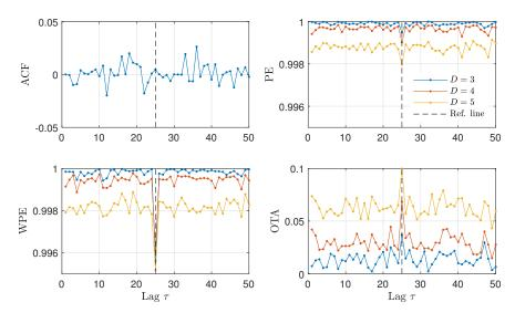
**Figure 3.** ACF and ordinal quantifiers estimated with several orders D as a function of the lag  $\tau$  ( $1 \le \tau \le 50$ ) for the NLMA model with feedback strength  $\alpha = 0.1$  and intrinsic time-delay  $\tau_0 = 25$ . Results obtained for a representative realization of length  $N = 10^4$  data are plotted.
