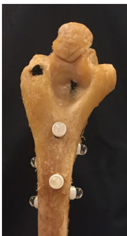
Figure A1. Image of the fully dissected specimen showing the posterior aspect of the humerus with glass spheres mounted on top of plastic hex-socket cap screws, which were screwed into the bone in step 1. Six spheres were fixed to the humerus (shown) and 6 to the ulna (not shown).
