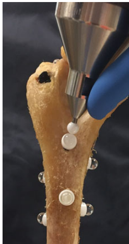
Figure A3. The specimen was locked at each flexion angle using a custom fixture, and the center of each sphere was identified using the digitizer with a ball probe affixed to its end.
