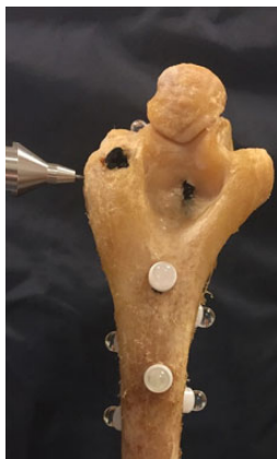
Figure A4. A point probe was affixed to the end of the digitizer and was used to identify the soft tissue and bony landmarks with the specimen fixed at 90° of flexion.
