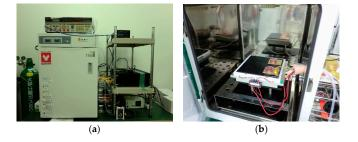
**Figure 1.** (a) The built-in incubator of the 0.12 THz exposure system, and (b) an inside view of the incubator. The cavity in the exposure system was maintained under controlled conditions similar to those in an incubator—i.e., an atmosphere of 95% air and 5%  $CO_2$  at a relative humidity of >95% and a temperature of 37 °C.
