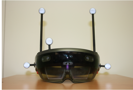
Figure 6. Rigid body affixed to the HoloLens device.
