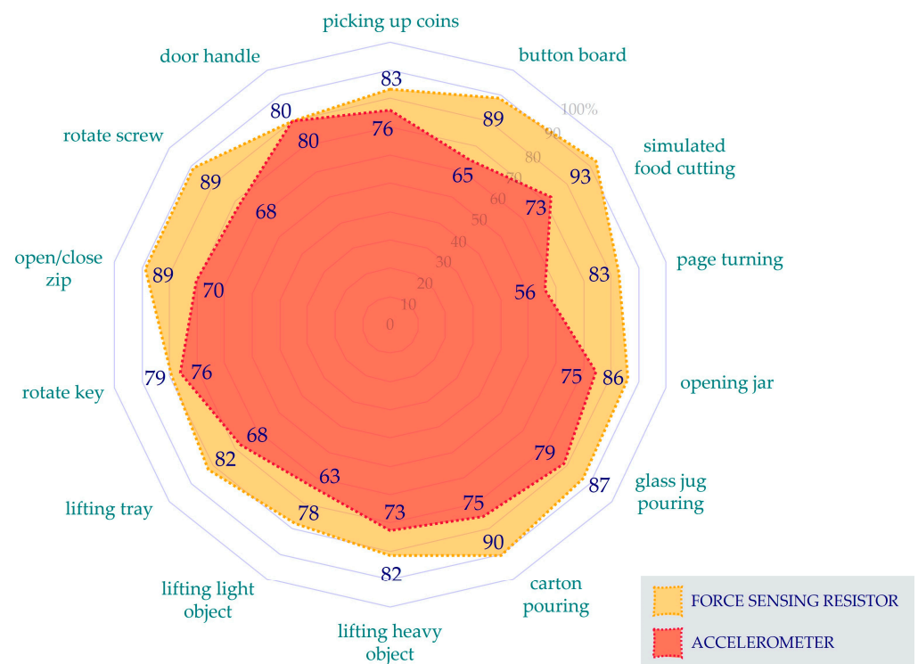
Figure 8. Average accuracy of wear time estimations, by the force sensing resistor (FSR) and accelerometer, whilst participants completed activities of daily living (ADLs) as part of the Southampton Hand Assessment Procedure (SHAP).
