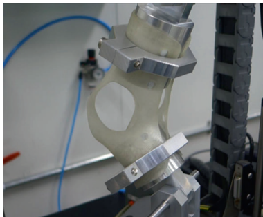
FIGURE 6: To evaluate the durability of the 3D-printed AFO, a mechanical stress test was performed. At both ends of the AFO orthosis made for the test, round-shaped plastic dummies were inserted and affixed to the machine.
