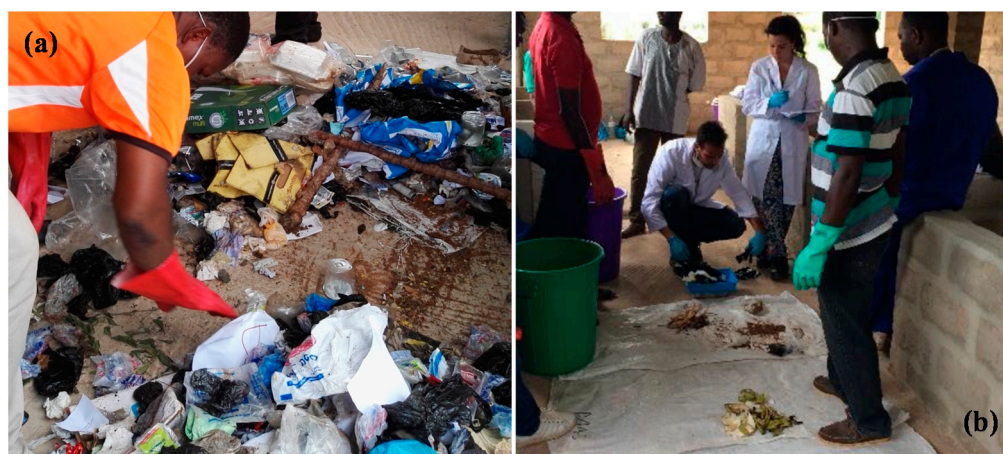
Figure 3. Laboratory work for urban solid waste characterization at the University of Lome. (a) Quartering and (b) weighing of some fractions after the separation.
