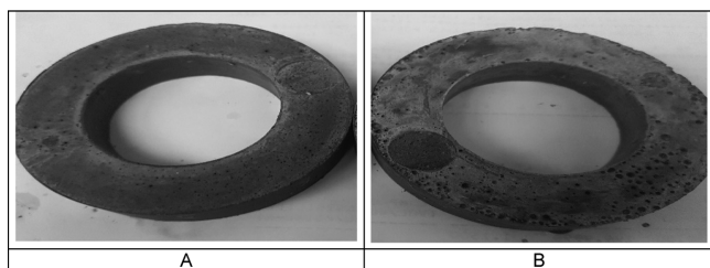
Figure 8. Samples from expansion molds, class G (A) and S-2 (B).
