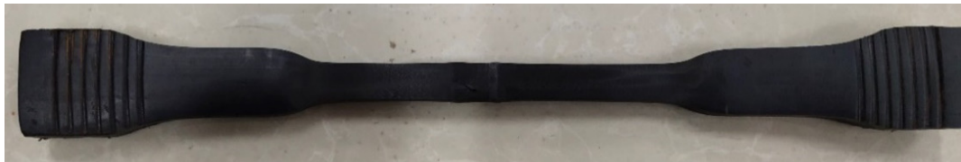
Figure 6. Creep failure specimen of HDPE without welding bead and welding defect under a load of 10 MPa and at a temperature of 28 °C.
