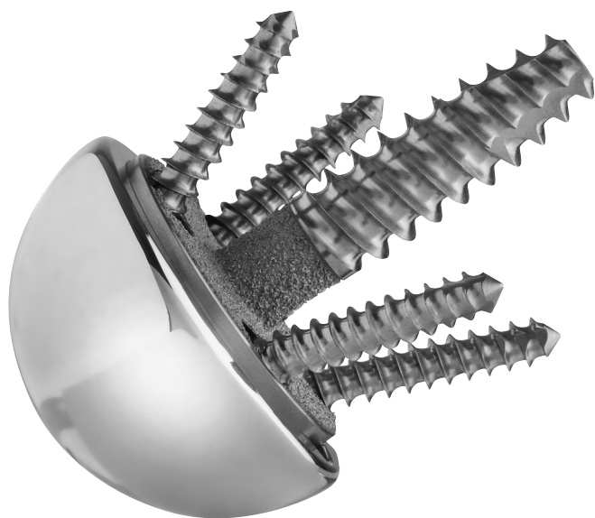
Figure 1 A monobloc baseplate with a hybrid central post, with a threaded uncoated medial portion and an unthreaded titanium plasma-sprayed lateral portion.
