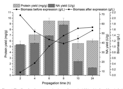
**Figure 1.** The effect of producer propagation time on the protein yield (mg/g) released from inclusion bodies, the NA yield (U/g) and on the amount of biomass (g/L) before and after NA gene expression.
