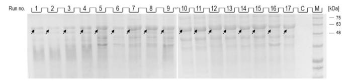
**Figure 3.** SDS-PAGE analysis of dissolved inclusion body fractions from individual optimization runs (1–17) and control (C). The position of the band corresponding to the recombinant NA in each lane is indicated by an arrow. Protein ladder indicates molecular weights in kDa (lane M).
