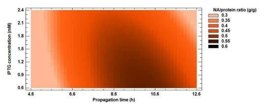
**Figure 5.** Response surface model plot showing the effect of IPTG concentration and propagation time on NA/protein ratio (g/g) at a constant optimized value of propagation time.
