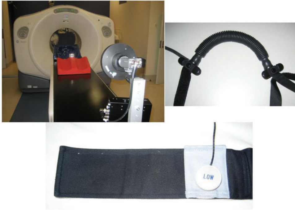
Figure 10 Varian RPM gating system (top left), Phillips Bellows (top right) and Anzil belt and pressure sensor (bottom).
