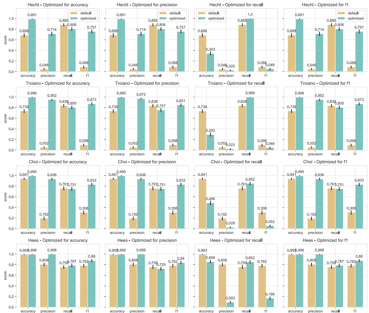
Figure 9. Classification performance as a result of hyperparameter tuning for accuracy, precision, recall, and F1 for Hecht, Troiano, Choi, and Hees. Each figure also shows the effect that optimizing for one metric has on the remaining metrics. For example, optimizing for recall results in a very low precision score for all four algorithms. Besides optimized scores, we also show the default classification scores obtained by using the default hyperparameter values for easy comparison; which can also be viewed in Fig. 4. Error bars indicate the 95% confidence interval.
