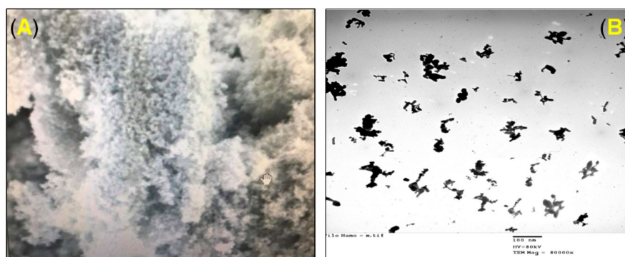
Figure 1. Scanning (SEM) (A), and transmission electron micrographs (TEM) (B) of synthesized zinc oxide nanoparticles (ZnO-NPs); 1–100 nm, HV = 80 kV, and TEM Mag = 8000×.
