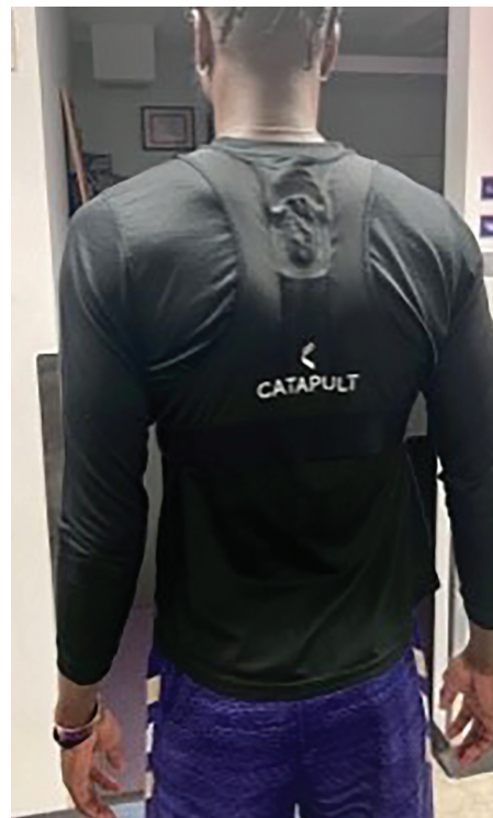
Figure 1. Wearable global navigation satellite system and local positioning system devices. The Catapult compression vest sits between the scapula with straps over the shoulders and underneath the axilla.
