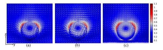
**Figure 2.** Electric field distributions in the yz plane at different peaks for 620 nm on glass substrate (a), LiNbO<sub>3</sub> substrate (b), and for 665 nm on Au film/glass substrate (c). The white arrows depict the electric field vector.
