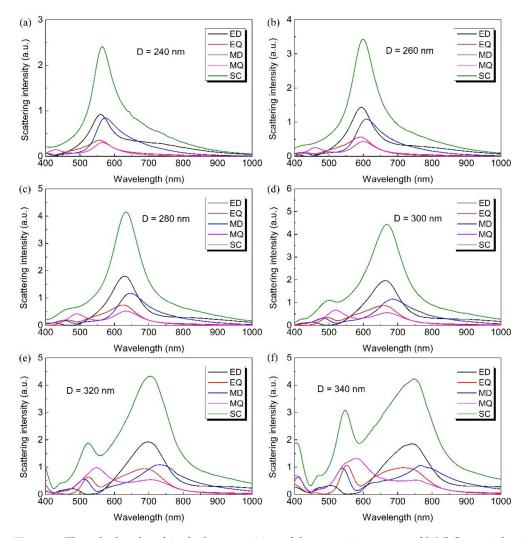
**Figure 4.** The calculated multipole decomposition of the scattering spectra of LiNbO<sub>3</sub> particle with diameters (**a**) D = 240 nm, (**b**) D = 260 nm, (**c**) D = 280 nm, (**d**) D = 300 nm, (**e**) D = 320 nm and (**f**) D = 340 nm on Au film/glass substrate.
