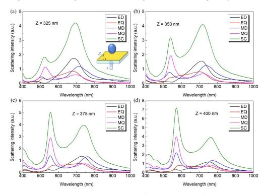
**Figure 6.** The calculated multipole decomposition of the scattering spectra for LiNbO<sub>3</sub> particle placed on 50 nm Au film/glass substrate with a fixed axis of 300 nm at in the xy directions and varying axis perpendicular to the Au film. Z represents the length of the particle in the z direction with (**a**) Z = 325 nm, (**b**) Z = 350 nm, (**c**) Z = 375 nm and (**d**) Z = 400 nm.
