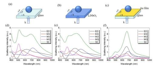
**Figure 1.** Schematic of LiNbO<sub>3</sub> particle with diameter D = 300 nm placed on a glass substrate (**a**), a LiNbO<sub>3</sub> substrate (**b**) and an Au film/glass substrate (**c**). The corresponding multipole decomposition of the scattering spectrum are displayed in the second row (**d**–**f**). SC represents the total scattering intensity.
