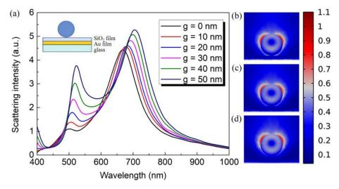
**Figure 5.** (a) The evolution of the scattering spectra for LiNbO<sub>3</sub> particle of diameter D = 300 nm placed on SiO<sub>2</sub> film/Au film/glass substrate with an increasing thickness (g) of SiO<sub>2</sub> layer, g = 0 nm, 10 nm, 20 nm, 30 nm, 40 nm, and 50 nm. (b–d) represent the electric field distribution in the yz plane for g = 10 nm at 670 nm, g = 30 nm at 690 nm, and g = 50 nm at 705 nm, respectively.
