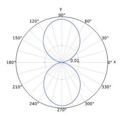
**Figure 3.** Radiation pattern in the xy plane for LiNbO<sub>3</sub> nanoparticles (D = 300 nm) placed on an Au film/glass substrate.
