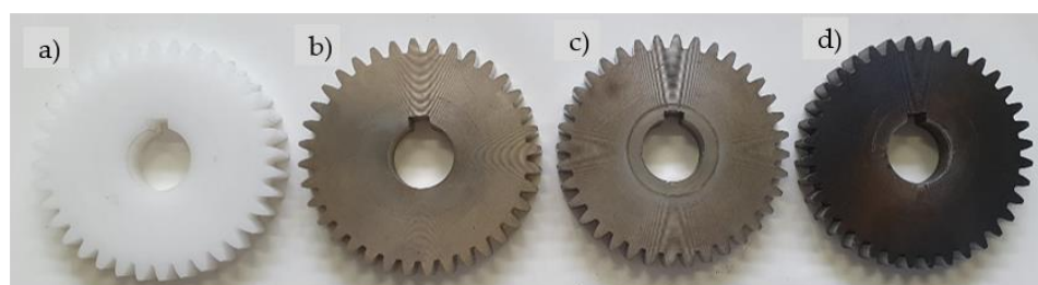
Figure 2. Tested gears made of POM: (a) without coating, (b) Al-coating, (c) Cr-coating, (d) CrN-coating.
