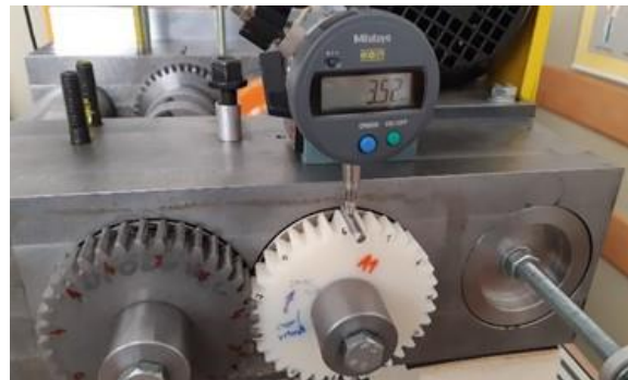
Figure 8. Measurement of the tooth thickness of a gear.
