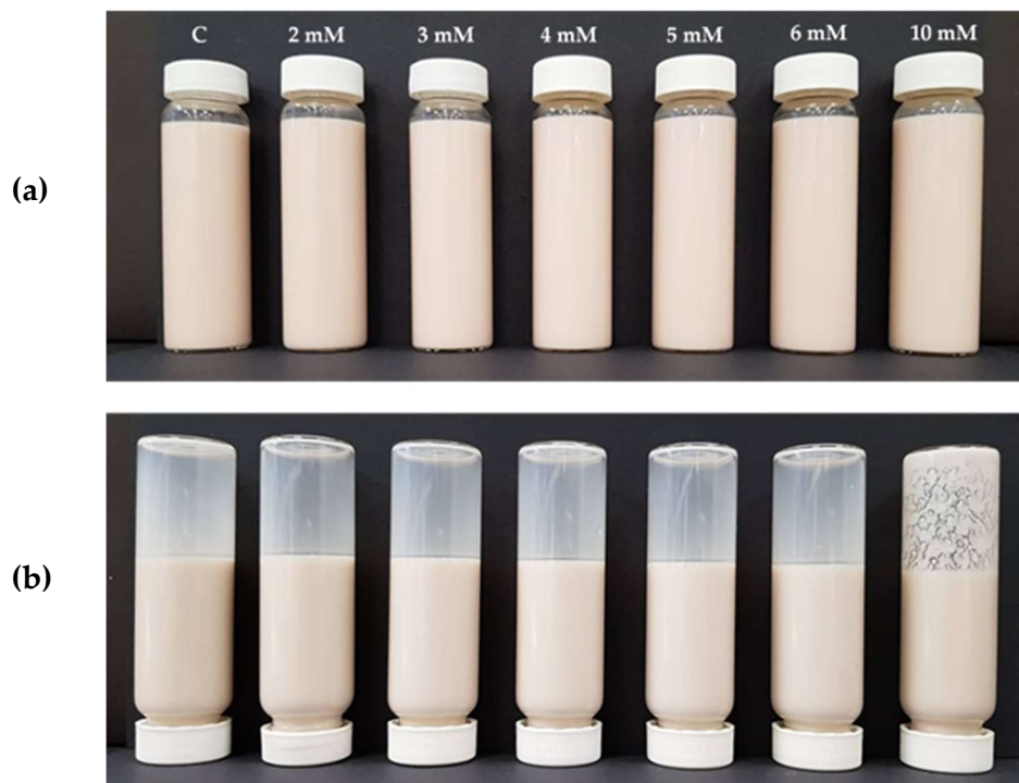
Figure 3. Photographs of lentil protein-stabilised emulsions containing 0 (C), 2, 3, 4, 5, 6, 10 mM calcium chloride before (a) and after (b) heat treatment at 95 °C for 30 s.
