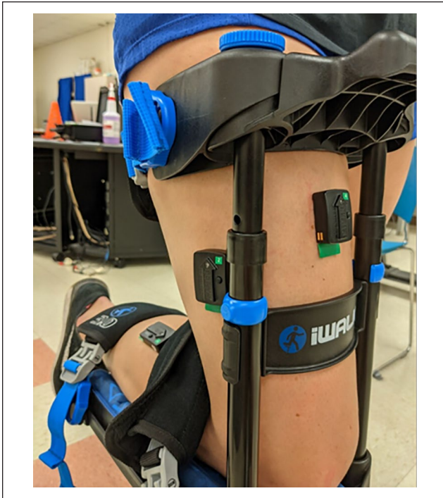
Figure 1. Trigno Avanti wireless Bluetooth sensors placement on a participant wearing the hands-free single crutch (iWALKFree). The left sensor is attached to the skin overlying the belly of the lateral gastrocnemius, the middle is over the belly of the vastus lateralis, and the right electrode is overlying the belly of the rectus femoris. The gluteus maximus sensor cannot be seen in this image.
