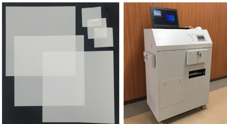
**FIG. 1.** The appearances of various size of the TLD-sheets (left) and the TLD reader (TLDR-1) (right). The TLD-sheet is white and semi-transparent. Data can be acquired using the TLDR-1 within 15 min.
