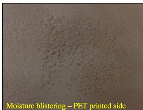
Figure 13. The blisters formed on the Ni ink film.
