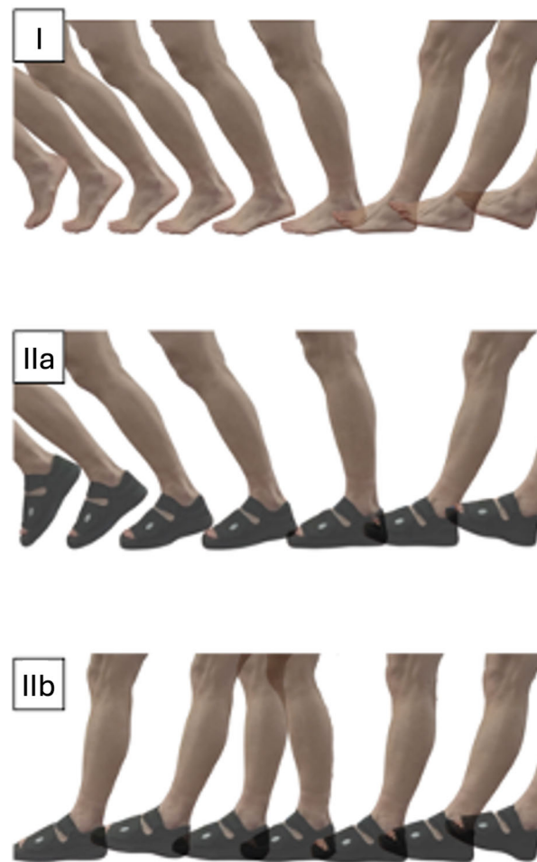
Figure 2. (I) Normal barefoot gait over a measuring plate placed on the track. (IIa) Normal gait in a POS with an inserted pressure measurement insole—putting weight on the whole foot. (IIb) Heel-accentuated “limping gait” in the POS without rolling over the entire foot.
