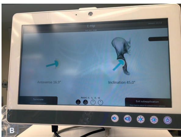
Figure 4. A. Implantation of the acetabular component with conventional cup applicator equipped with holder (white arrow) for measuring sensor (black arrow). Reference sensor (black arrowhead). B. Monitor with real-time information on acetabular component position.
