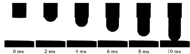
FIGURE 11. Example of an HSV image sequence of an indenter strike with an object distance of 3 mm and a spring compression distance of 3.5 mm. An average indenter velocity of 3.0 m/s can be derived.
