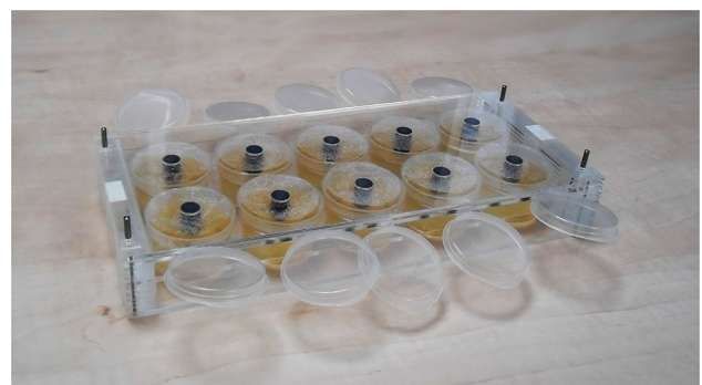
FIGURE 16. The mold for creating the environment models. The mold consists of laser-cut disks in between which 10 circular containers can be placed. The lid of the mold, in which several rods are placed, creates the notches.
