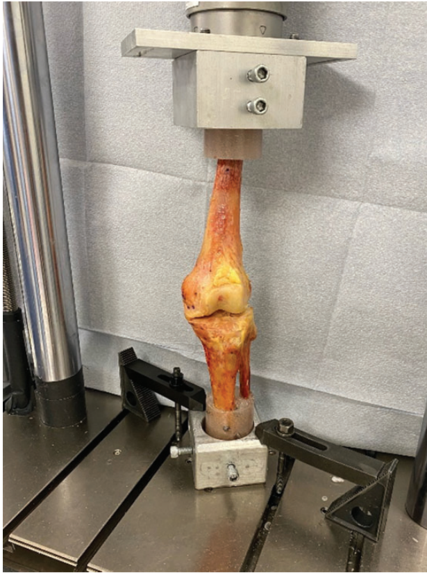
Figure 4. Specimen mounted in actuator before pull-to-failure biomechanical testing.
