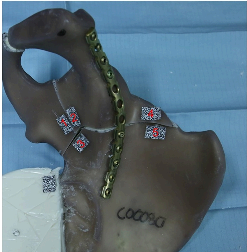
Fig 4. Shows the standardized placement of the spackle patterns. Four different fracture gap displacements were measured. The optical measurement was performed between spackle pattern 1/2, 1/3, 2/3 and 4/5 (1 = os ischii; 2 and 4 = os pubis; 3 and 5 = os ilium).
