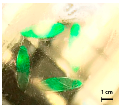
Figure 7. Photography of four holographic reflection gratings daylight illuminated.
