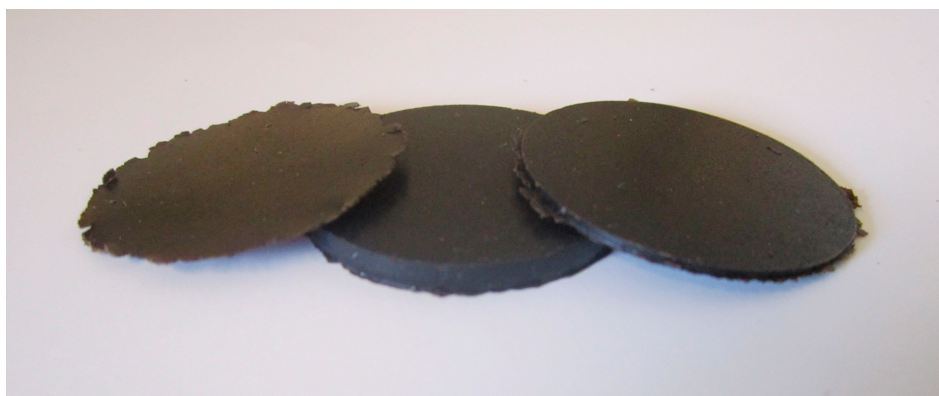
Figure 1. Compression-molded plates/films of the larva material (diameter: 35 mm, thickness from left to right: 180 \mu\text{m} , 3 mm and 1 mm).
